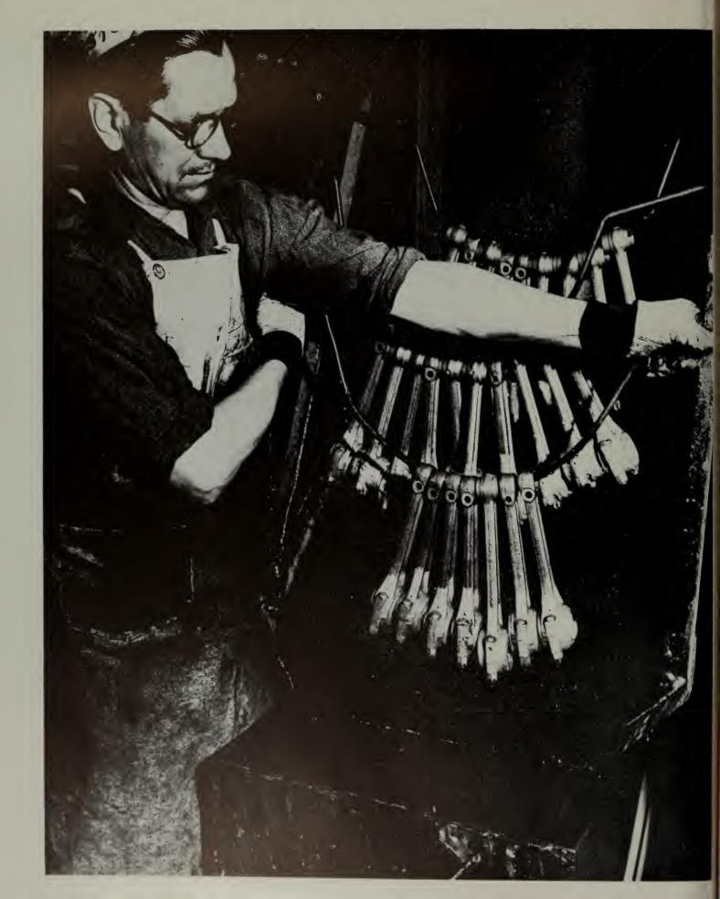
The rods are now dipped in a rust preventative and are then hung on a rack to dry,—as shown in above picture.
